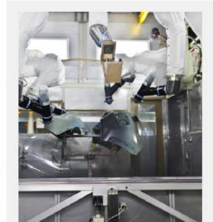
Toyota's Canadian assembly plant in Cambridge, Ontario, developed a new cleaning agent to clean the robots in the paint booth between colors. The new solvent/water mix uses 43,000 liters (11,300 gallons) less solvent than the previous version and reduces the number of bumpers that need to be recycled in half.
